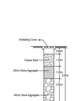
Cross Section Of Rain Water Harvesting Well
